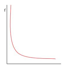
The above plot shows that the limiting stress 'f' decreases as increases. In fact, when very small, limiting stress is is close to infinity, which is not rational. Limiting stress cannot be greater than the yield stress of the material.
