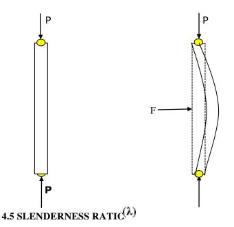
Slenderness ratio is defined as the ratio of effective length ( $l_e$ ) of the column to the minimum radius of gyration (r min) of the cross section.
