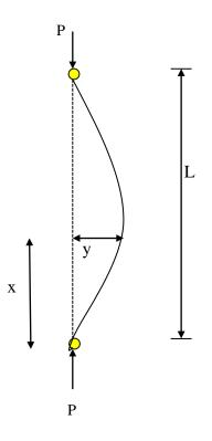
Consider a section at a distance x from the origin. Let y be the deflection of the column at this section. Bending moment in terms of load P and deflection y is given by
