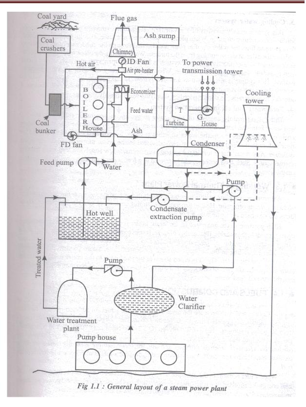
**3.** *Feed water and steam circuit:* The prime mover develops power by utilizing steamGenerated in the boiler. Then a condenser is used to condense the steam coming out of prime mover and a pump is used to feed the condensate to the boiler. In the boiler shell and tubes, water circulation is setup due to density difference of waterbetween low and high temperature sections. A super heater is used to super heat the wetsteam from boiler drum and is then supplied to the prime movers.
