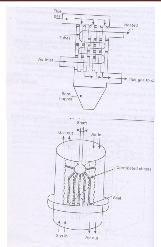
It consists of series of tubes through which the combustion gases pass with air passing around the outside of the tubes. The combustion gases transfer heat to the air and heated this preheated air is supplied to the furnace. The baffle plates deflect the direction of
