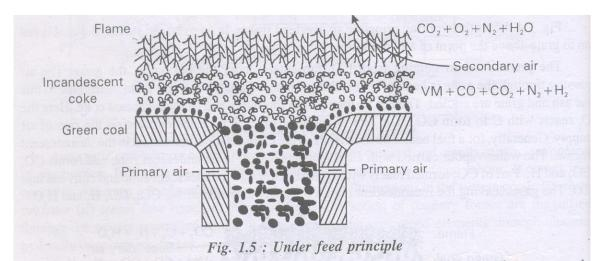
In this type, the coal is admitted in to the furnace below the point of air admission. ie., bothcoaland air moves in the same direction. This type is suitable for burning the semibituminous and bituminouscoals.
