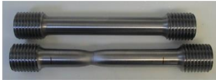
Necking in Tensile specimen
