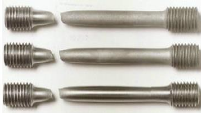
Necking in Tensile specimen
