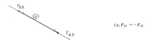
Since link 3 is acted upon by only two forces,  $F_{43}$  and  $F_{23}$  are collinear, equal in magnitude and opposite in direction
