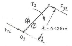
Link 2 is acted upon by 2 forces and a torque (stated in the problem), for equilibrium the two forces must be equal, parallel and opposite and their sense must oppose  $T_2$ .
