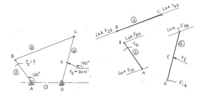
Link 3 is acted upon by only two forces  $F_{23}$  &  $F_{43}$  and they must be collinear & along BC. Link 4 is acted upon by three forces  $F_{14}$ ,  $F_{34}$  &  $F_{4}$  and they must be concurrent. LOA  $F_{34}$  is known and  $F_{E}$  completely given.
