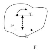
For equilibrium, the two forces must form a counter couple. Therefore the forces must be equal, opposite and parallel and their senses must be so as to oppose the couple acting on the body
