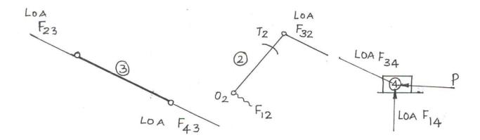
Force triangle for the forces acting on  $\bigcirc$ 4 is drawn to some suitable scale. Magnitude and direction of P known and lines of action of  $F_{34}$  &  $F_{14}$  known.
