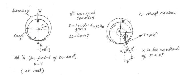
While rotating, the point of contact shifts to B; R<sup>n</sup> passes through B.
