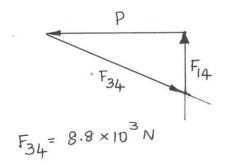
Measure the lengths of vectors and multiply by the scale factor to get the magnitudes of  $F_{14}$  &  $F_{34}$ . Directions are also fixed.
