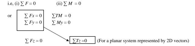
Fx, Fy, Fz force Components along X, Y & Z axis
