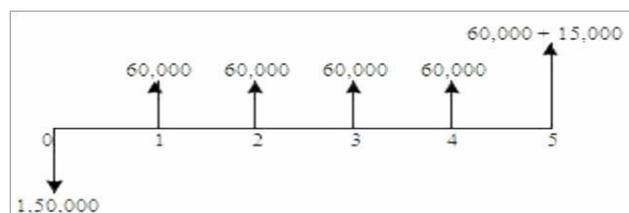
**Fig. 3.7** Cash flow diagram for alternative A
