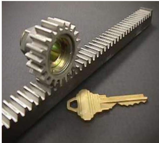
Figure: Steel gear and rack cut with an abrasive water jet
