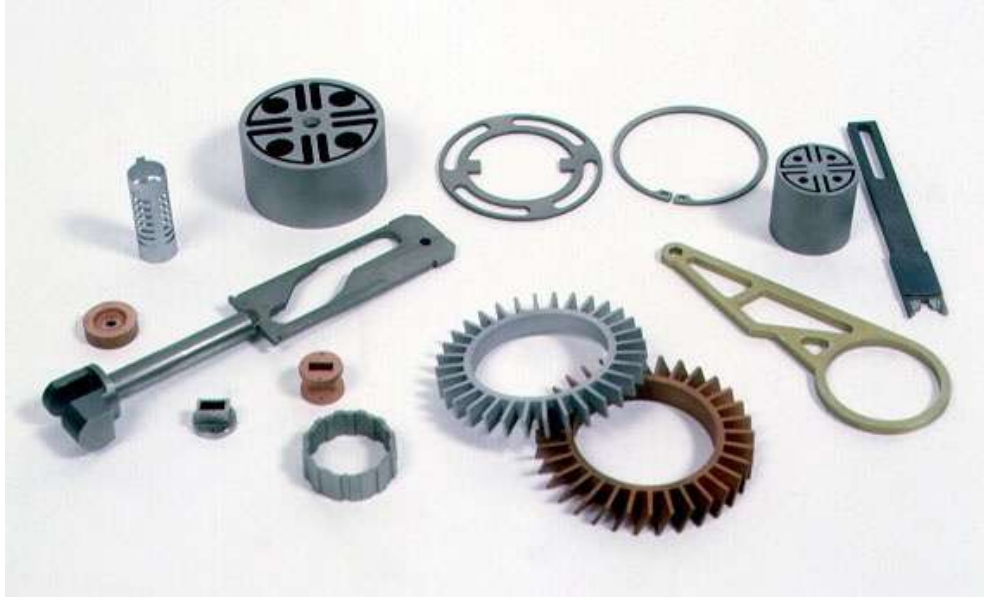
Figure: Difficult internal parts made by EDM process
