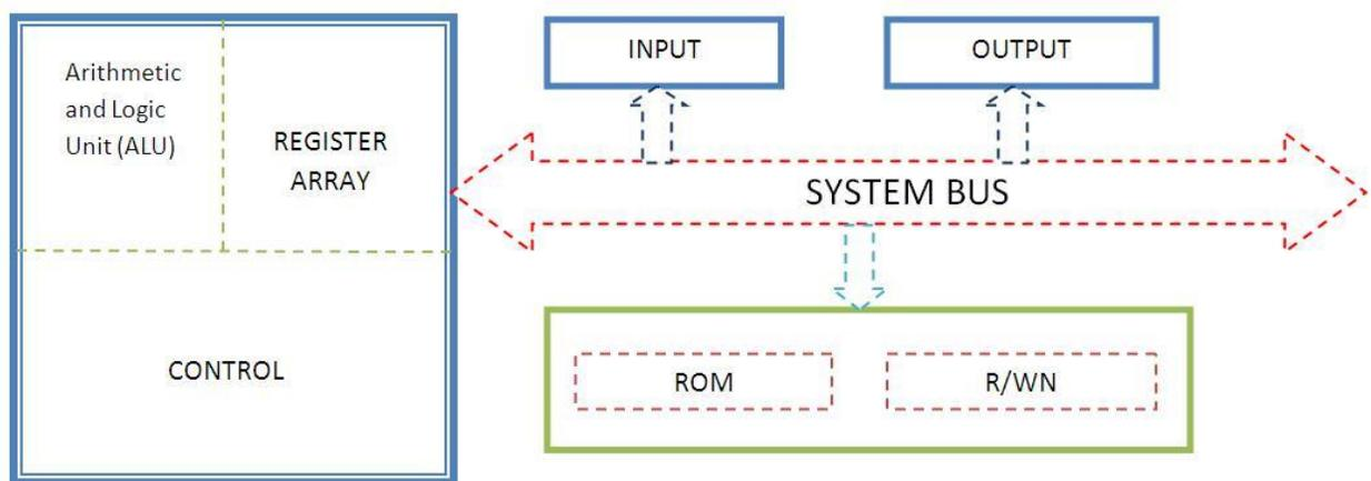
Figure 2 Schematic of configuration of a micro processor
