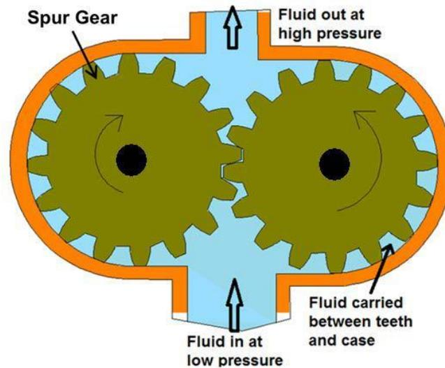
Fig. 5.3.4 Gear motor
