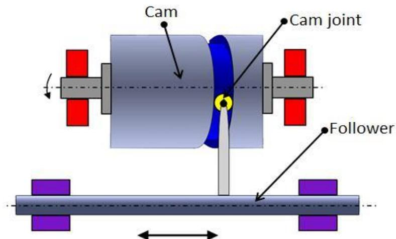
Figure 4.3.4 Cylindrical cam
