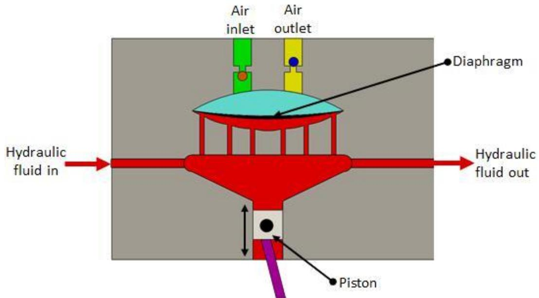
Fig. 5.1.1 Diaphragm compressor
