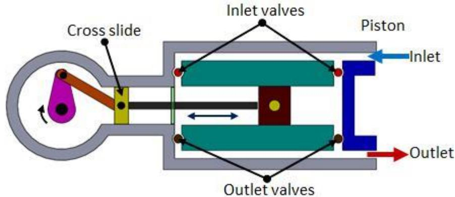
Fig. 5.6.4 Double acting piston compressor
