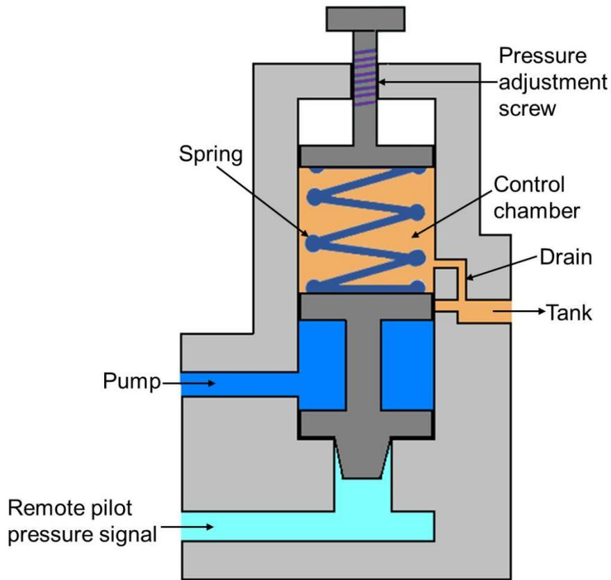
Figure 5.2.27 Unloading Valve
