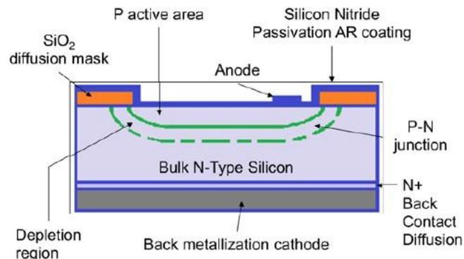
Fig 2: Construction of Photo diodes
