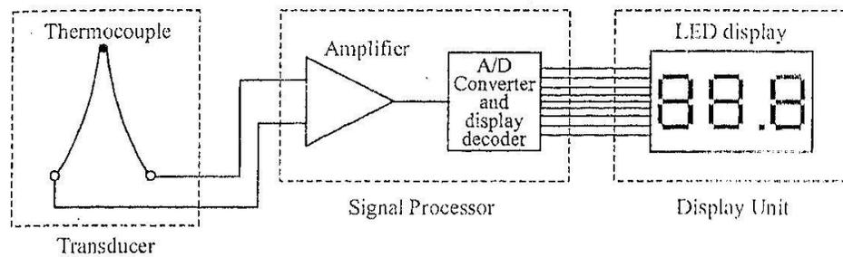
Fig 3: Digital thermometer principle
