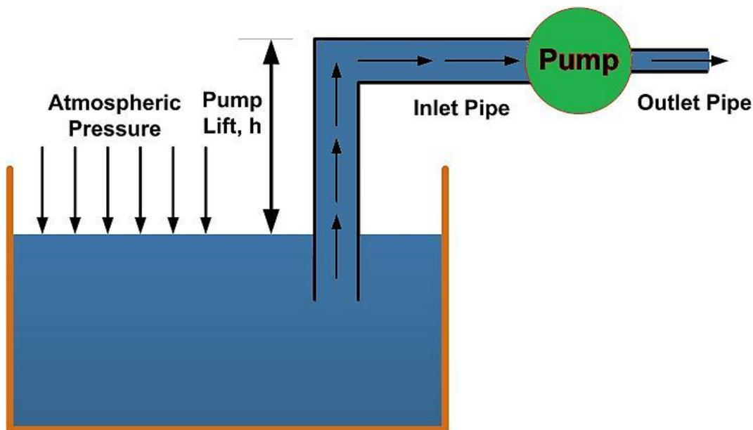
Figure 5.4.4 Pump lift
