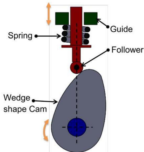
Figure 4.3.1 Cam mechanism.
