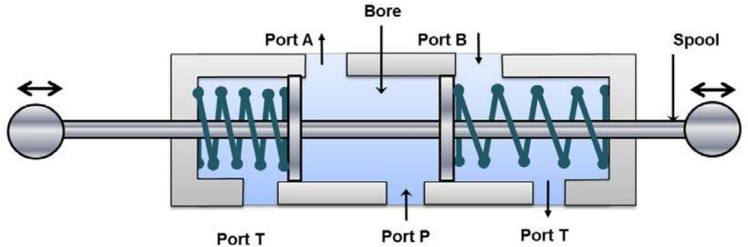
Figure 5.2.11 Three position four way valve: P to A and B to T
