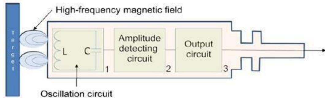
Fig 3: Construction of Eddy current proximity sensors
