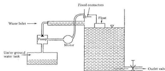
Fig 7: Water level controller
