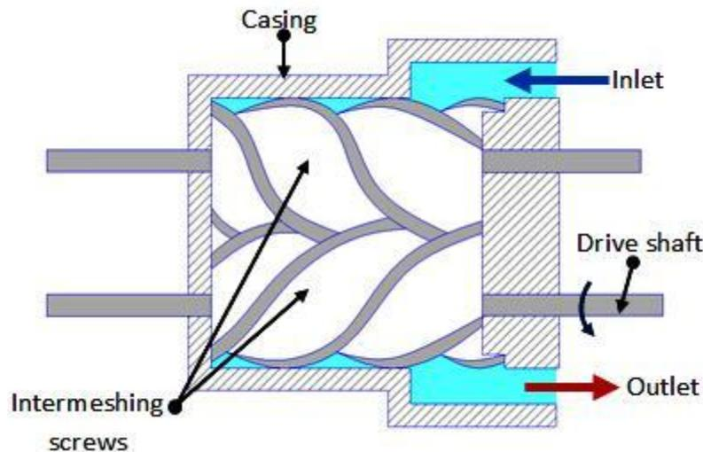
Fig. 5.1.2 Screw compressor
