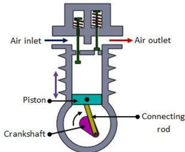
Fig. 5.6.3 Single acting piston compressor
