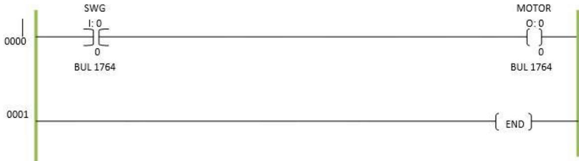
Figure 3.3.5 A rung to run the conveyer belt.
