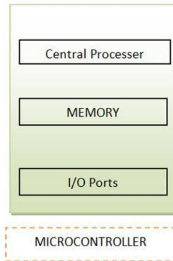
Figure 4 Schematic of microcontroller.
