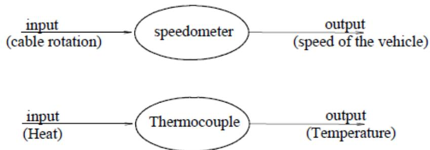
figure: concept of measurement
