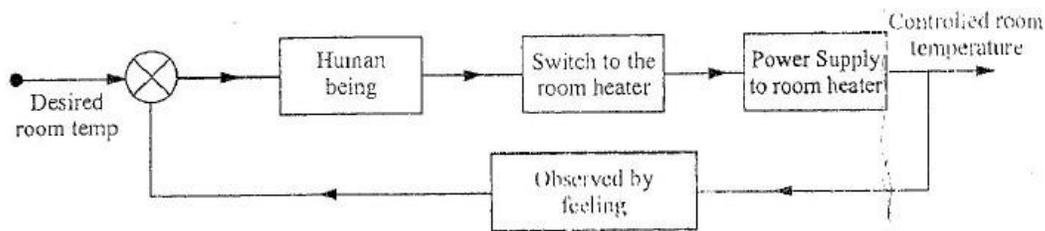
Fig 8: Room Temperature Controller
