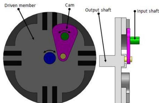
Fig. 4.5.4 Internal Geneva mechanism
