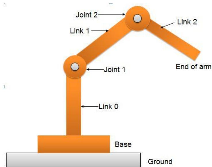
Fig. 3.5.1 Joint-link scheme for robot manipulator
