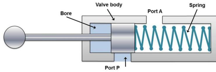
Figure 5.5.1 Valve closed
