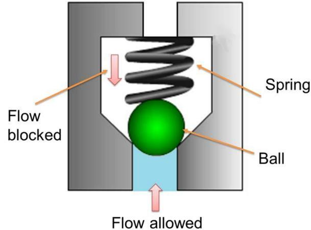
Figure 5.2.1 Inline check valve
