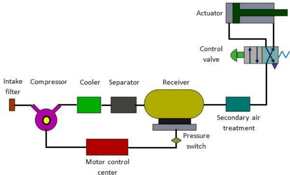
Fig. 6.1.1 Components of a pneumatic system
