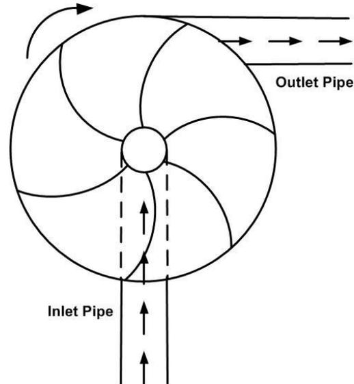
Figure 5.4.3 Centrifugal pump
