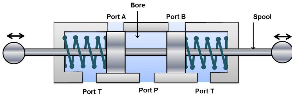
Figure 5.2.12 Three position four way valve: closed center
