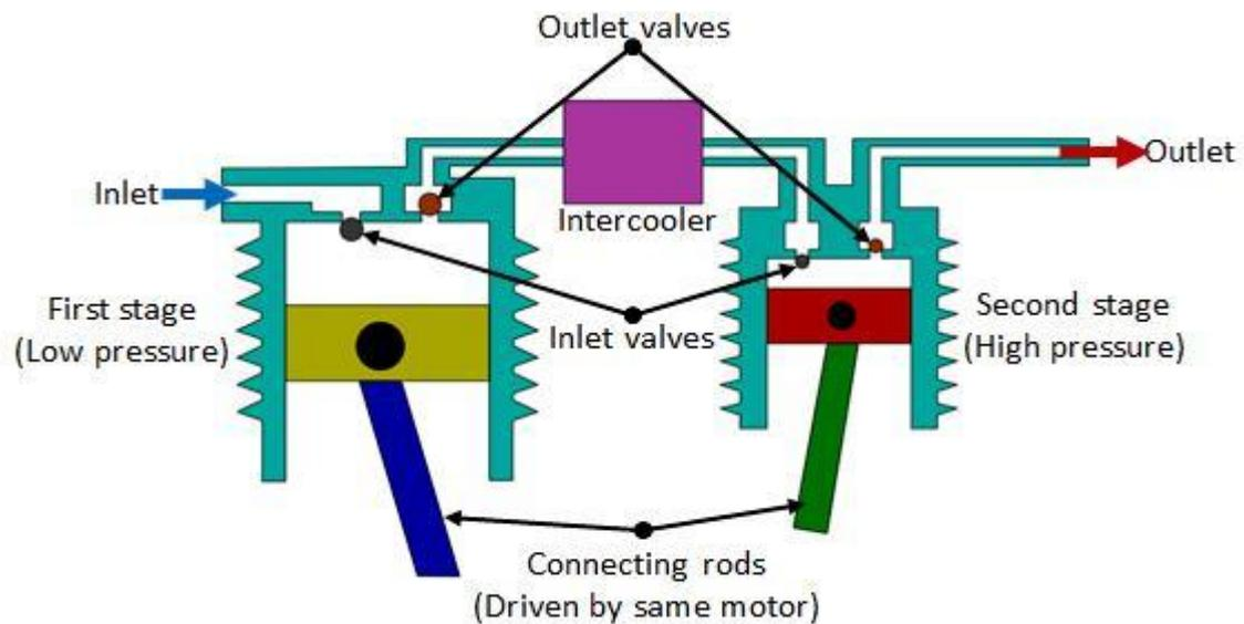
Fig. 6.1.5 Multi-stage compressor
