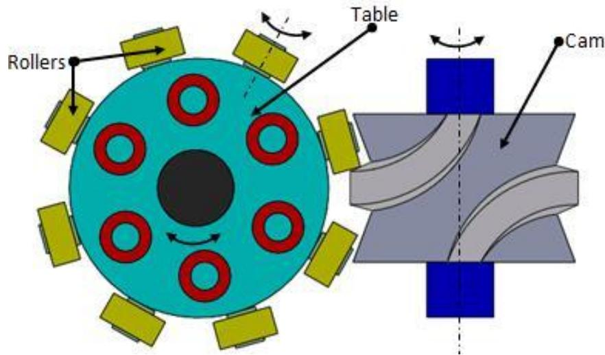
Fig. 4.5.6 Cam mechanism
