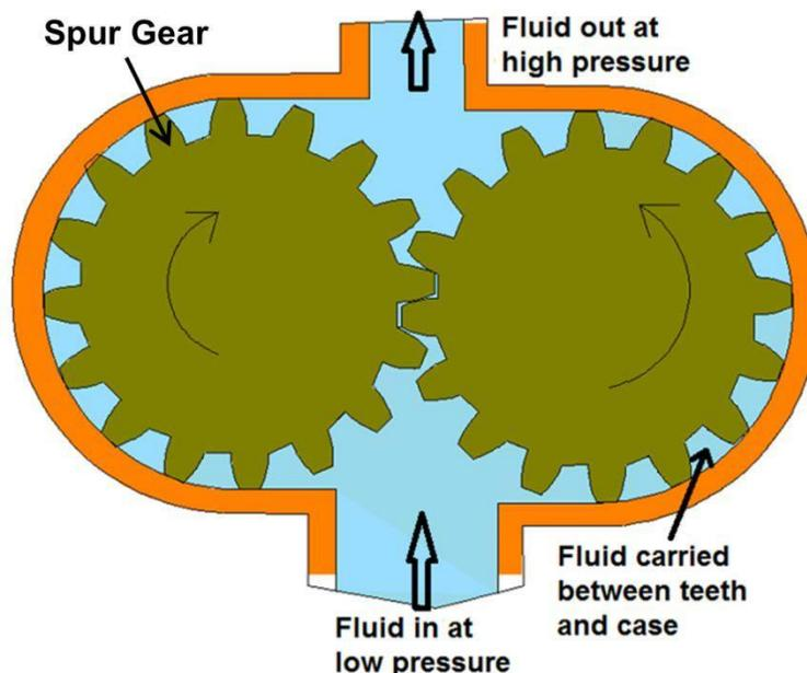
Figure 5.2.1 Gear pump
