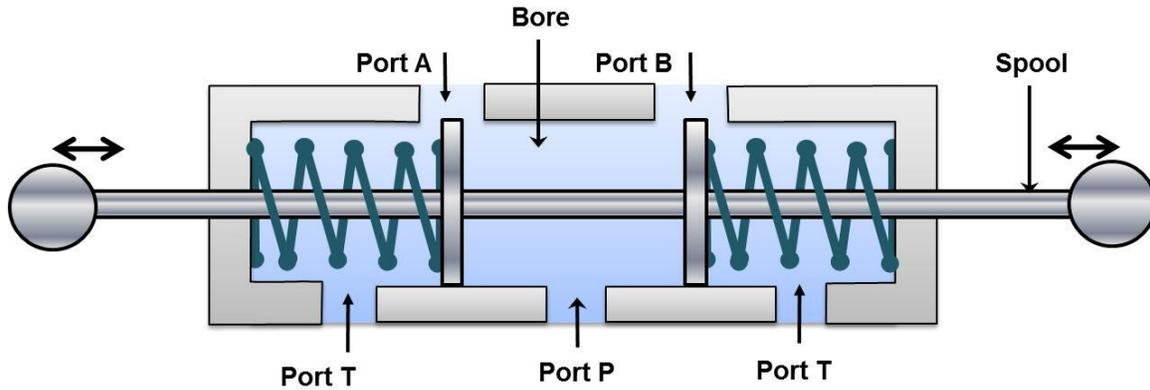
Figure 5.2.9 Three position four way valve in open center mode
