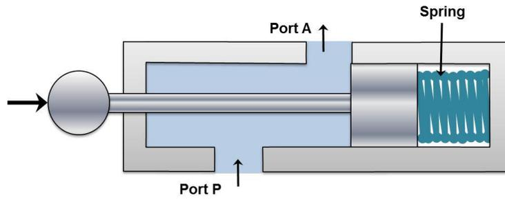
Figure 5.5.2 Valve opened by actuation
