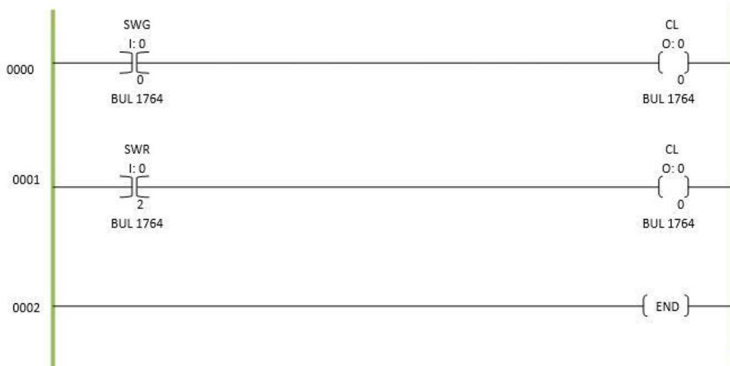
Figure 3.3.6 Program code to actuate a pneumatic cylinder
