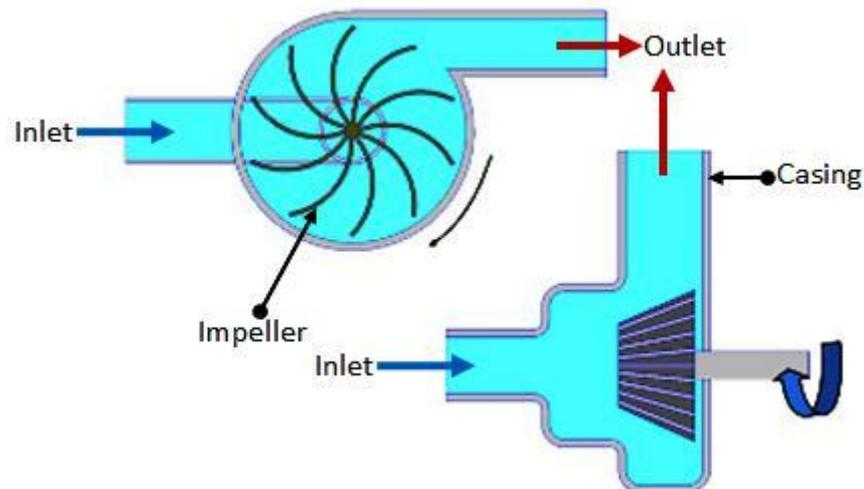
Fig. 5.1.6 Blower (Centrifugal type)
