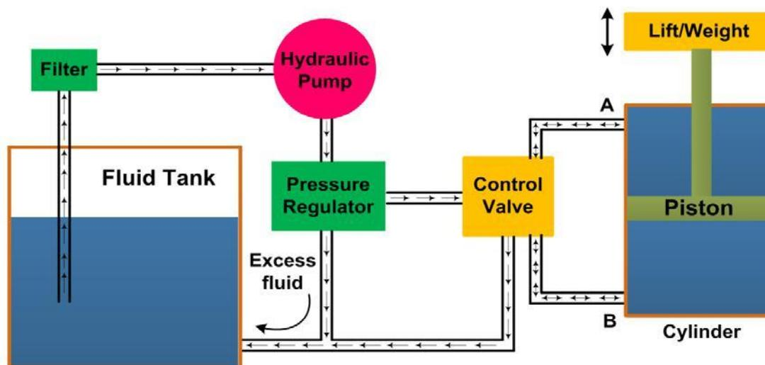
Figure 5.4.2 Schematic of hydraulic system
