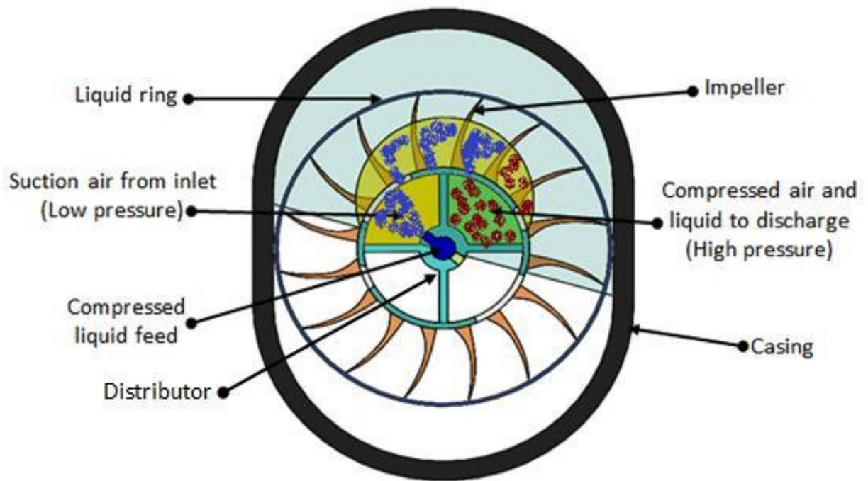
Fig. 5.1.4 Liquid ring compressor
