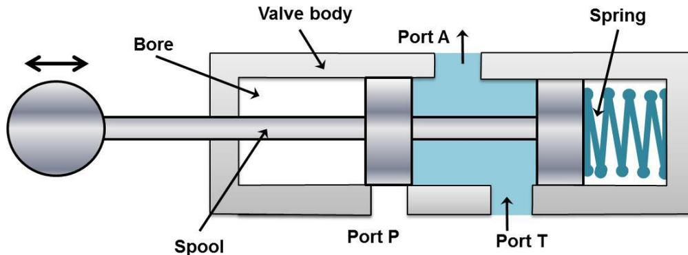
Figure 5.2.8 Three way valve in closed position
