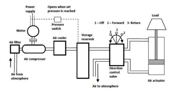
Pneumatic systems have components that are similar to those used in hydraulic systems.
