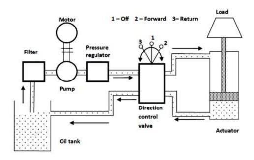
There are six basic components required in a hydraulic system:
