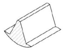
3. *T-ring seal:* T-ring seal is a dynamic seal that is extensively used to seal cylinder-pistons, piston rods and other reciprocating parts. It is made of synthetic rubber moulded in the shape of the cross-section T and reinforced by backup rings on either side. The sealing edge is rounded and seals very much like an O-ring.
