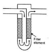
**2. Proportional filters (bypass filters):** In some hydraulic system applications, only a portion of oil is passed through the filter instead of entire volume and the main flow is directly passed without filtration through a restricted passage.
