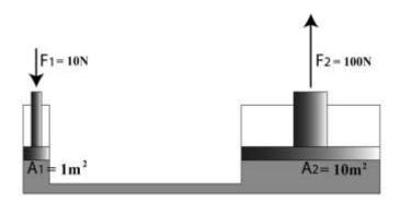
The above figure shows how Pascal's law can be applied to produce a useful amplified output force. Consider an input force of 10N is applied to a 1-m<sup>2</sup> area piston. This develops a  $10\text{N/m}^2$  pressure throughout the oil within the housing. This  $10\text{N/m}^2$  pressure acts on a  $10\text{-m}^2$  area piston producing a 100N output force. This output force performs useful work as it lifts the 100N weight.
