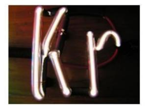
A krypton-filled discharge tube in the shape of the element's atomic symbol. A colorless, odorless, tasteless noble gas, krypton occurs in trace amounts in the atmosphere, is isolated by fractionally distilling liquefied air. The high power and relative ease of operation of krypton discharge tubes caused (from 1960 to 1983) the official meter to be defined in terms of one orange-red spectral line of krypton-86.
