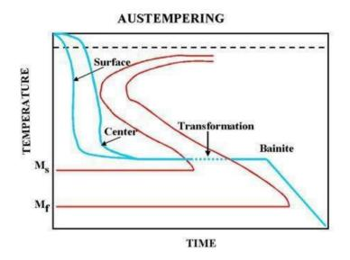
Bainite structure have stenghts slightly lower than martensitic structure,but
