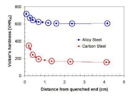
To illustrate the use of jominy test result in the selection of steels, consider the hardenability curve for two diff steels shown in the fig above.
