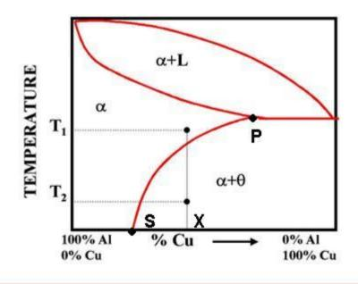
a) Solutiontreatment solution treatment involves heating the certain temperature that causes the alloying atoms to dissolve into the section. This results in a homogeneous solid solution of single phase.
