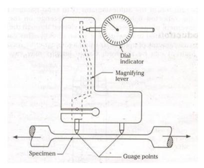
Mechanical Strain Gauge (Berry Extensometer)
