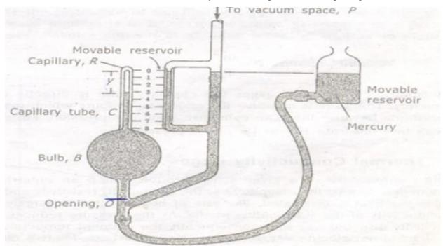
The Bulb B and capillary tube C are then at the same pressure as that of the vacuum pressure P. The reservoir is subsequently raised until the mercury fills the bulb and rises in the capillary tube to a point where the level in the reference capillary R is located at the zero point. If the volume of the capillary tube per unit length is 'a' then the volume of the gas in the capillary tube is Vc = ay----(1).
