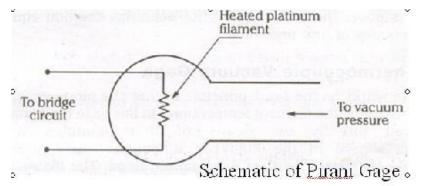
To measure the resistance of the filament wire a resistance bridge circuit is used. The usual method is to balance the bridge at some datum pressure and use the out-of-balance currents at all other pressures as a measure of the relative pressures.
