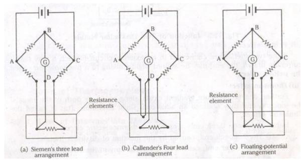
Methods of Compensating Lead Resistance Error
