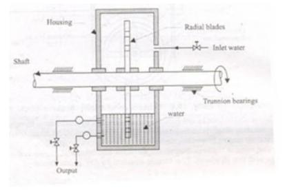
Fig. Section through a typical water brake
