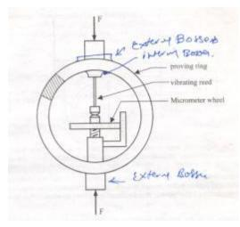
The deflection is small and hence the usefulness of the proving ring as a calibration device depends on the accuracy with which this small deflection is measured. This is done by using a precision micrometer shown in the figure. In order to obtain precise measurements one edge of the micrometer is mounted on a vibrating reed device which is plucked to obtain a vibratory motion. The micrometer contact is then moved forward until a noticeable damping of the vibration is observed.
