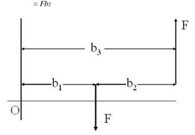
The important reason for measuring torque is to obtain load information necessary for stress or deflection analysis. The torque T may be computed by measuring the force F at a known radius 'r' from the following relation T=Fr.
