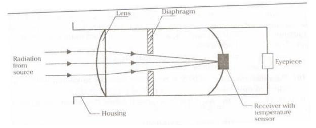
Schematic of Lens Type Radiation Receiving Device
