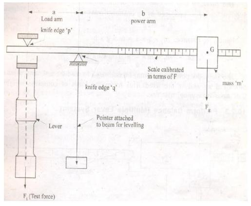
Fig. Schematic of Unequal Arm Balance
