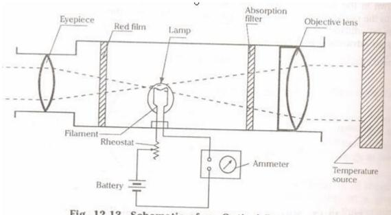
Fig. 12.13 Schematic of an Optical Pyrometer
