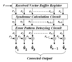
Fig. 4.13 General Decoding scheme for an (n,k) linear block code
