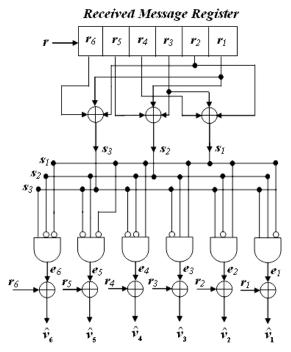
Fig 4.14: Decoding circuit for (6,3) code
