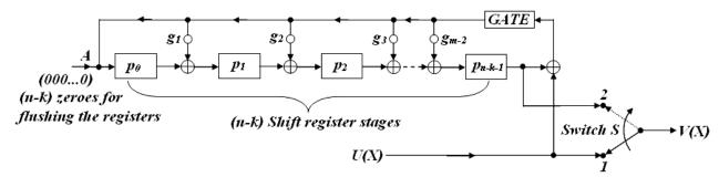
Fig 4.8 Syndrome encoding of cyclic codes using (n-k) shift register stages
