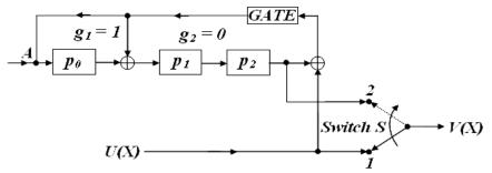
Fig 4.9 Encoder for the (7,4) cyclic code
