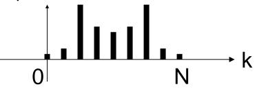
$$H(e^{j\omega}) = \sum_{k=0}^{N} h[k]e^{-j\omega . k} = \dots = e^{-j\omega L} \sum_{k=0}^{L} a_k \cos(\omega k)$$
