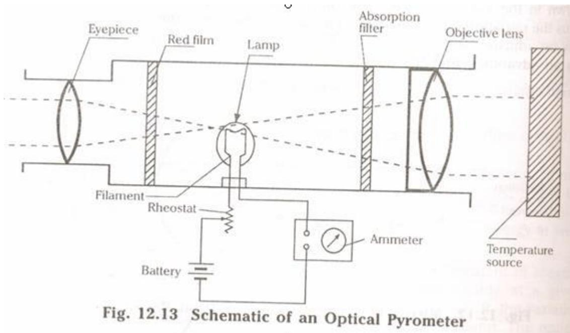
The eyepiece is then adjusted such that the filament and the source appear superimposed. The filament may appear either hotter or colder than the unknown source as shown in the Fig. The current through the filament is adjusted by means of rheostat.
