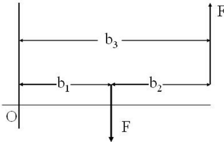
The important reason for measuring torque is to obtain load information necessary for stress or deflection analysis. The torque T may be computed by measuring the force F at a known radius 'r' from the following relation  $T=Fr$ .
