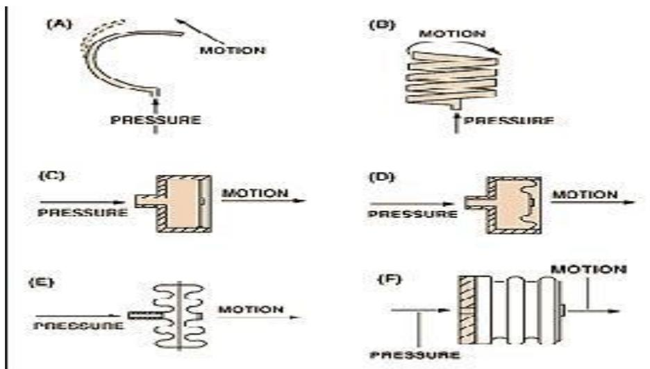
The basic pressure sensing element can be configured as a C-shaped Bourdon tube (A); a helical Bourdon tube (B); flat diaphragm (C); a convoluted diaphragm (D); a capsule (E); or a set of bellows (F).
