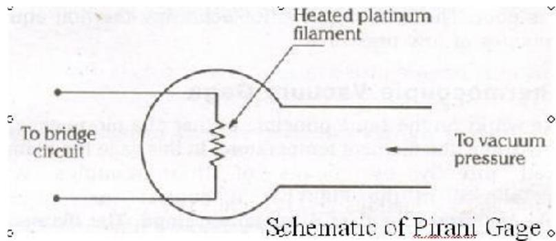
To measure the resistance of the filament wire a resistance bridge circuit is used. The usual method is to balance the bridge at some datum pressure and use the out-of-balance currents at all other pressures as a measure of the relative pressures.
