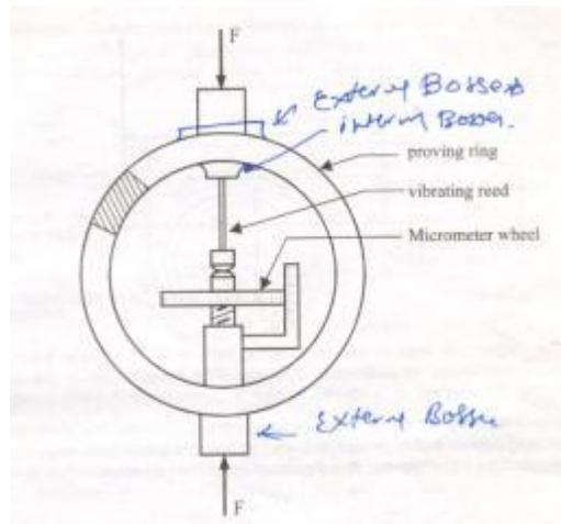
The deflection is small and hence the usefulness of the proving ring as a calibration device depends on the accuracy with which this small deflection is measured. This is done by using a precision micrometer shown in the figure. In order to obtain precise measurements one edge of the micrometer is mounted on a vibrating reed device which is plucked to obtain a vibratory motion.
