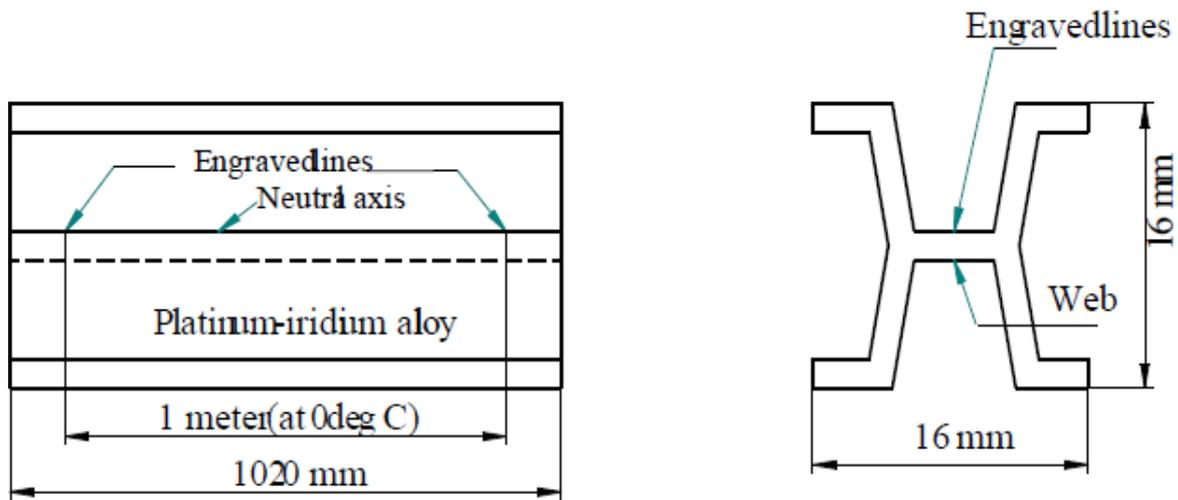
The tresca cross section gives greater rigidity for the amount of material involved and is therefore economic in the use of an expensive metal. The platinum-iridium alloy is used because it is non oxidizable and retains good polished surface required for engraving good quality lines.
