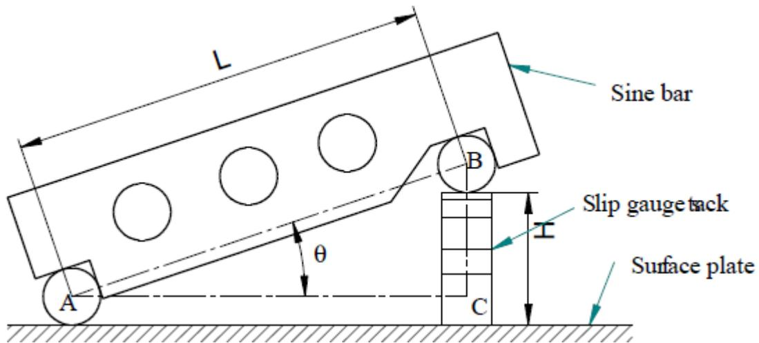
**(1) For checking unknown angles of a component**
