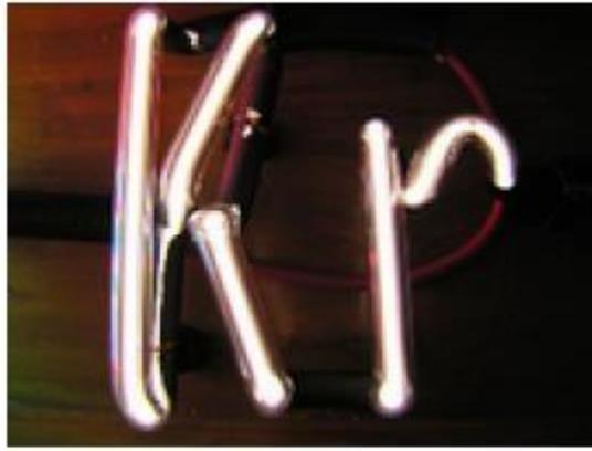
A krypton-filled discharge tube in the shape of the element's atomic symbol. A colorless, odorless, tasteless noble gas, krypton occurs in trace amounts in the atmosphere, is isolated by fractionally distilling liquefied air. The high power and relative ease of operation of krypton discharge tubes caused (from 1960 to 1983) the official meter to be defined in terms of one orange-red spectral line of krypton-86.
