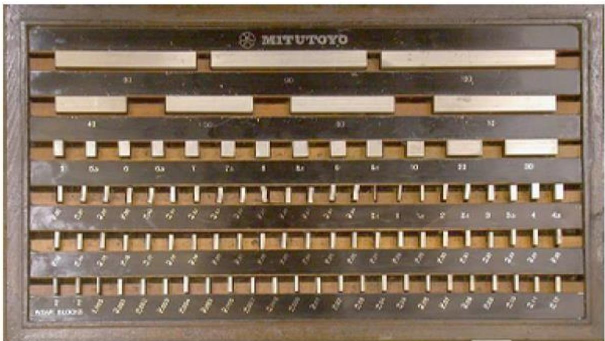
Slip gauges are blocks of steel that have been hardened and stabilized by heat treatment. They are ground and lapped to size to very high standards of accuracy and surface finish. A gauge block (also known Johansson gauge, slip gauge, or Jo block) is a precision length measuring standard consisting of a ground and lapped metal or ceramic block. Slip gauges were invented in 1896 by Swedish machinist Carl Edward Johansson.
