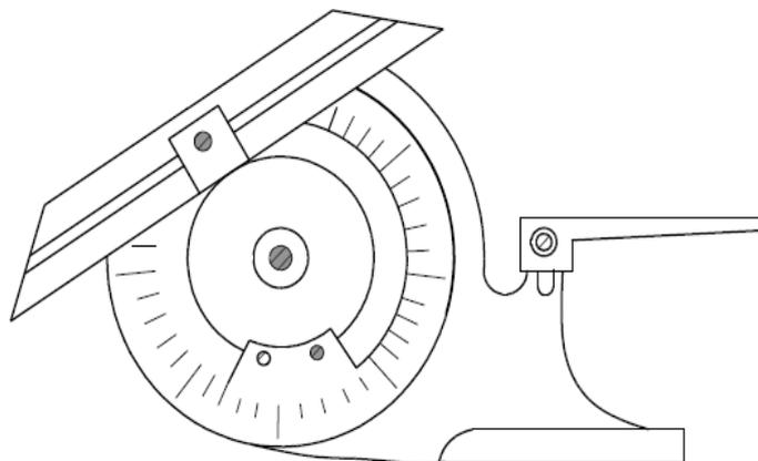
The adjustable blade is capable of sliding freely along the groove provided on it and can be clamped at any convenient length. The adjustable blade along with the circular plate containing the vernier can rotate freely about the center of the main scale engraved on the body of the instrument and can be locked in any position with the help of a clamping knob.
