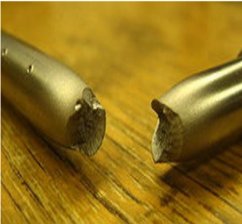
1 Ductile failure of a specimen strained axially. 2 Schematic representation of the steps in ductile fracture (in pure tension).
