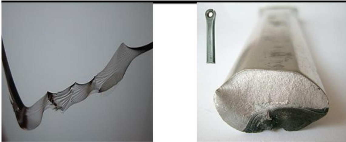
1 Brittle fracture in glass 2. Fracture of an aluminum crank arm. Bright: brittle fracture. Dark: fatigue fracture
