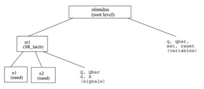
Figure 2-6. Design Hierarchy for SR Latch Simulation
