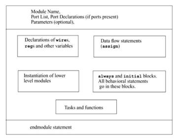
Figure 2.2.:Components of a Verilog Module
