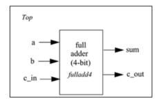
Figure 2-4. I/O Ports for Top and Full Adder
