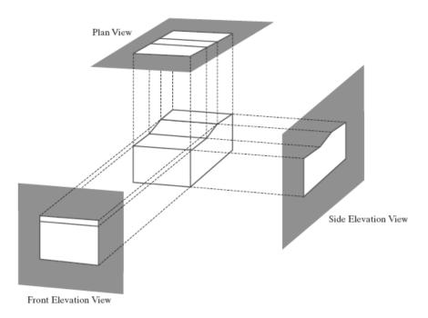
➔ Front, side, and rear orthogonal projections of an object are called *elevations;* and a top orthogonal projection is called a *plan view*
