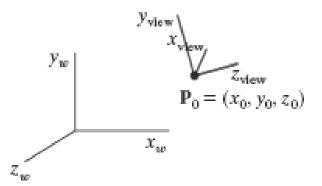
A right-handed viewing-coordinate system, with axes x <sub>view</sub>, y <sub>view</sub>, and z <sub>view</sub>, relative to a right-handed worldcoordinate frame.
