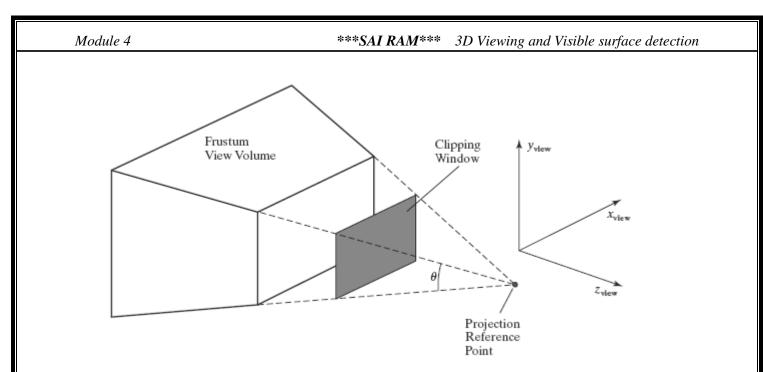
✓ For a given projection reference point and view-plane position, the field-of view angle determines the height of the clipping window from the right triangles in the diagram of Figure below, we see that
