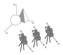
✓ Alternatively, different views of an object or group of objects can be generated using geometric transformations without changing the viewing parameters
