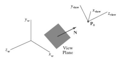
✓ An additional scalar parameter is used to set the position of the view plane at some coordinate value  $z_{vp}$  along the  $z_{view}$  axis,
