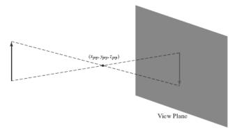
✓ Perspective effects also depend on the distance between the projection reference point and the view plane, as illustrated in Figure below.
