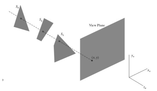
Figure above shows three surfaces at varying distances along the orthographic projection line from position (x, y) on a view plane.
