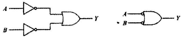
Bubbled OR gate and NAND gate are equivalent
