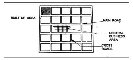
2) Radial or star and block pattern: In this, roads radially emerge from the central business area in all directions and between two built-up area will be there. The main advantage in this, central place is easy accessible from all the directions. E.g.: Nagpur
