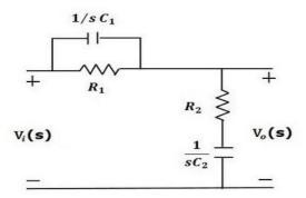
This circuit looks like both the compensators are cascaded. So, the transfer function of this circuit will be the product of transfer functions of the lead and the lag compensators.
