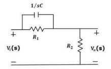
Here, the capacitor is parallel to the resistor  $R_1$  and the output is measured across resistor  $R_2$ . The transfer function of this lead compensator is –
