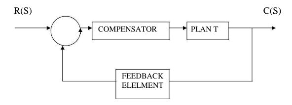
Lead compensation essentially yields an appropriate improvement in transient resonse and a small imrovement in steady state accuracy. Lag compensation on the other hand, yields an appreciable improvement in steady state accuracy ast the expense of increasing theh transient responsetime. Lag- lead compensation combines the characterisites of both lead compensation and lag compensation. The use of a lag- lead compensator raises the order of the system by two
