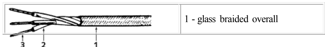
e) Braided circular insulated with glass fibre - Fig 4.2e
