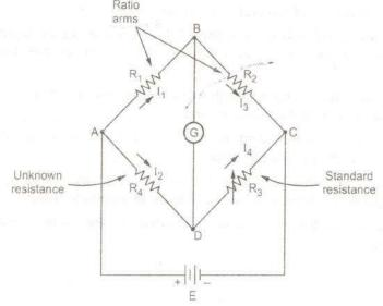
The arms consisting the resistances R] and R2 are called ratio arms. The arm consisting the standard known resistance R3 is called standard arm. The resistance R4 is the unknown resistance to be measured. The battery is connected between A and C while galvanometer is connected between Band D.
