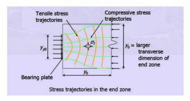
Bursting force: A portion of a pre-stressed member surrounding the anchorage is the end block.
