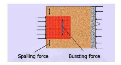
Fbst for an individual square end zone loaded by a symmetrically placed square bearing plate according to Cl 18.6.2.2 is,
