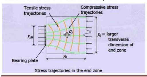
The larger transverse dimension of the end zone is represented as yo. The corresponding dimension of the bearing plate is represented as ypo. For analysis, the end zone is divided into a local zone and a general zone.
