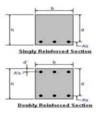
Rectangular Reinforced concrete beam
