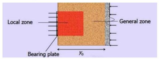
The local zone is the region behind the bearing plate and is subjected to high bearing stress and internal stresses. The behavior of the local zone is influenced by the anchorage device and the additional confining spiral reinforcement.
