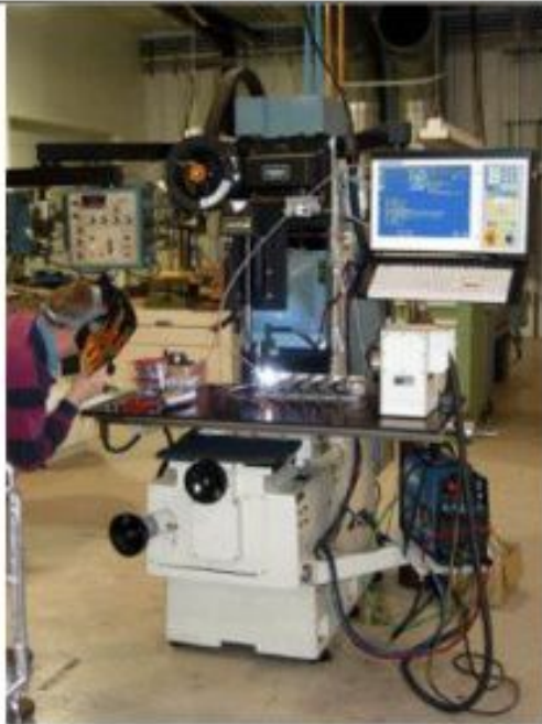
Figure 21.6 4 axis CNC Tig welding machine
