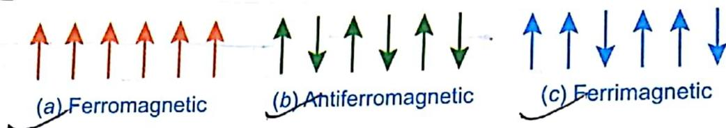
Fig. 1.20: Schematic alignment of magnetic moments
